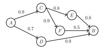
For every pair of directly connected nodes, say i and j, there is a given probability  $p_{ij}$  that the link from i to j is up. It is generally of interest to calculate the probability that there is a path connecting A and B in which all links are up.
